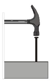
The mass of the hammer is 0.75 kg and its velocity, just before it hits the nail, is 15.0 m/s downward. After hitting the nail, the hammer remains in contact with it for 0.1 s. After this time both the hammer and the nail have stopped moving.
