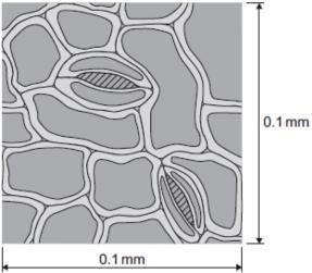
The length and width of this piece of leaf surface are both 0.1 mm.
