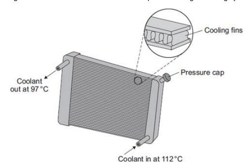
Liquid coolant, heated by the car engine, enters the radiator. As the coolant passes through the radiator, the radiator transfers energy to the surroundings and the temperature of the coolant falls.
