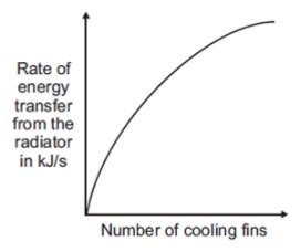
The number of cooling fins affects the rate of energy transfer from the radiator.
