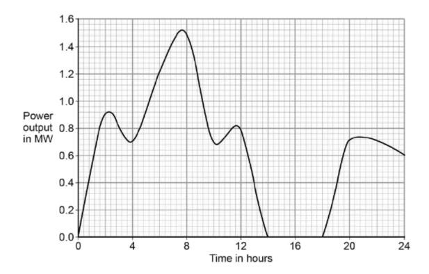
A wind turbine does not generate electricity constantly.
