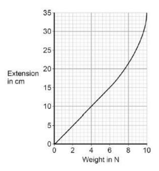
Use **Figure 3** to determine the additional force needed to increase the extension of the spring from 5cm to 15cm.
